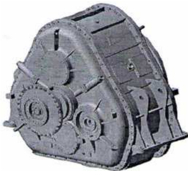
Figure 10. Photo of prototype of ship's gear reducer.
