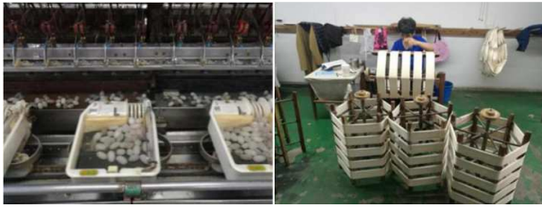
Figure 4. Automatic silk reeling and silk quality detection.
