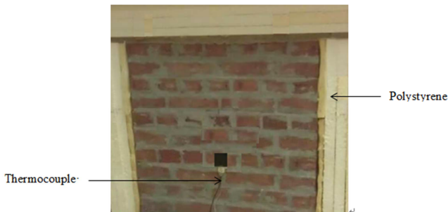
Figure 3. Experimental setup of the wall and insulation.
