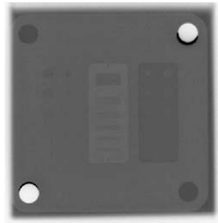
X-ray image (radiography) of the JSGI phantom.
