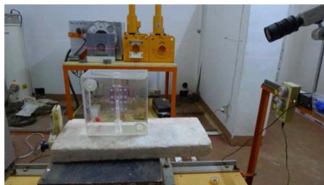
Figure 2. Irradiation of TLDs at SSDL (INSTN-Madagascar).
