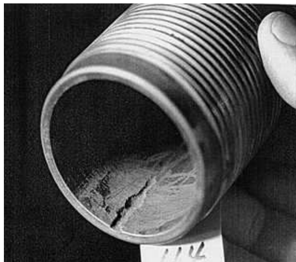
Figure 1. Wirelining damage leading to localized corrosion. From Reference 10.
