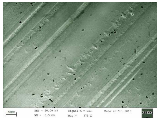
Figure 2(c). FESEM image of \text{LaMnO}_3 nanofibers at 700 °C
