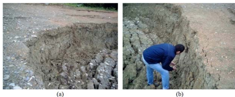
Figure 13. Two rotation landslides on the marl-filled layers.
