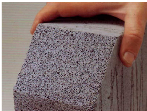
Figure 5. Penetrating internal structure appearance (pores).
