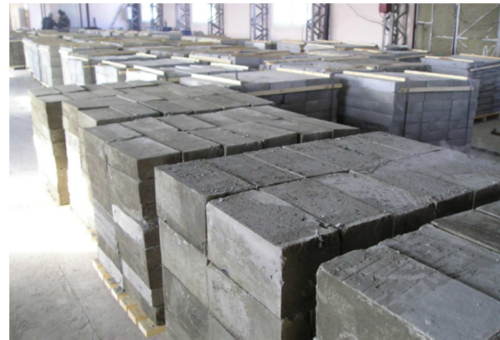
Figure 7. The finished product is penobetone. Dimensions 200x300x600mm.
