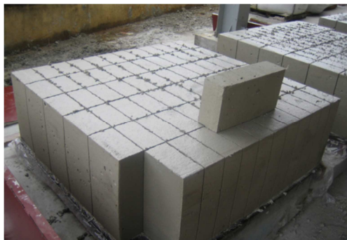
Figure 6. The finished product is penobetone. Dimensions-100x300x600mm.
