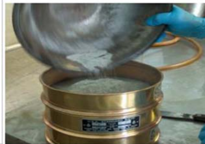
Figure 2. Pycnometer and Sieve Analysis.
