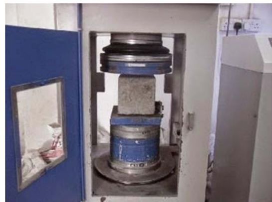
Figure 4. Compressive strength test on CTM.
