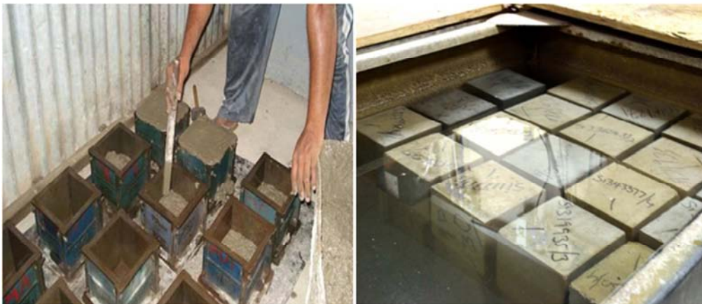
Figure 3. Showing casting and curing of cube.
