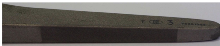
Figure 1. Prosthetic surface after anti-infective coating with spraying technique. Dark-grey represents coated areas, light-grey uncoated areas.
