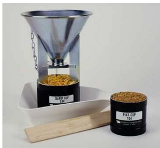
Figure 17. Measuring cup and cox funnel for bulk density.
