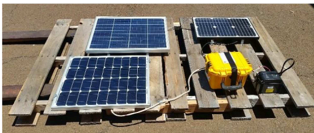
Figure 2. Test system with monocrystalline PV panel (lower left), polycrystalline panel (upper left), battery (black, lower right), weatherized case (yellow, lower right) and charging panel (upper right).
