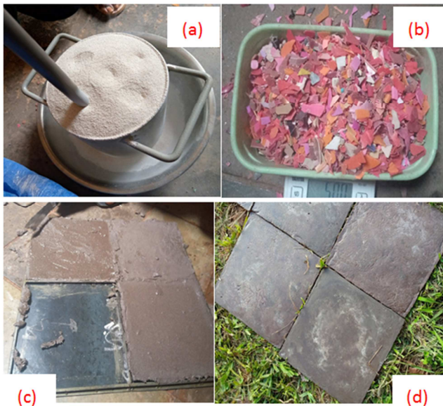
Figure 4. a) Eggshell powder; b) PPW; c) Tiles in mould; d) Manufactured floor tiles.
