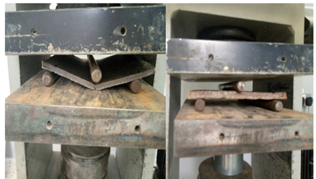
Figure 5. Performing flexural strength test using UTM.
