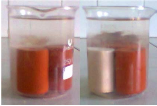
Figure 8. Water Absorption Capacity Tests specimen immersed in water for 28days.
