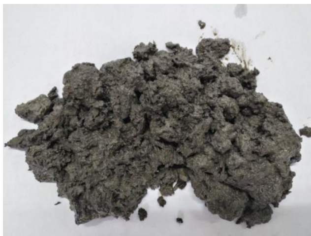
Figure 2. Emulsified asphalt Blended Directly with Cement for Demulsification and Losing the Workability.
