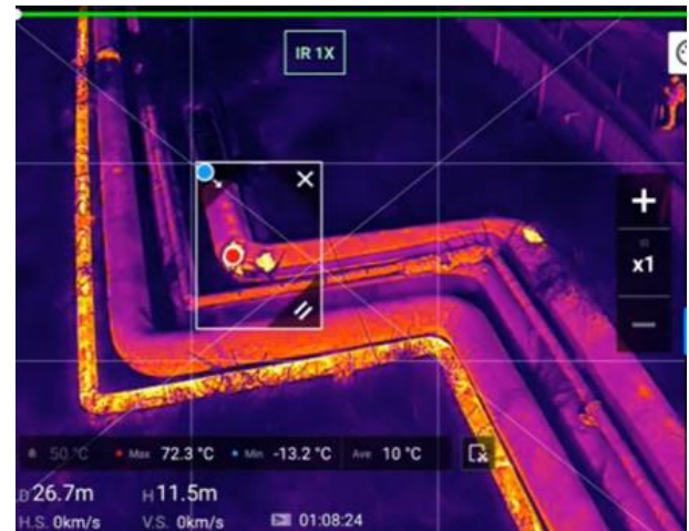
Figure 1. Infrared detection using a drone, the placement of heat energy loss.
