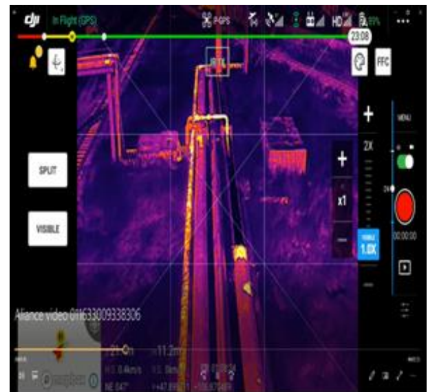
Figure 2. Infrared detection of damaged areas of thermal insulation.
