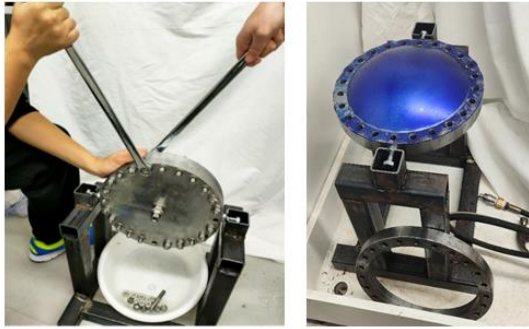
(a) Disassembly of the free-bulge forming set.
