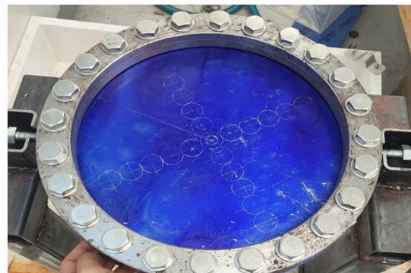
(b) Free-bulge forming set after assembly.
