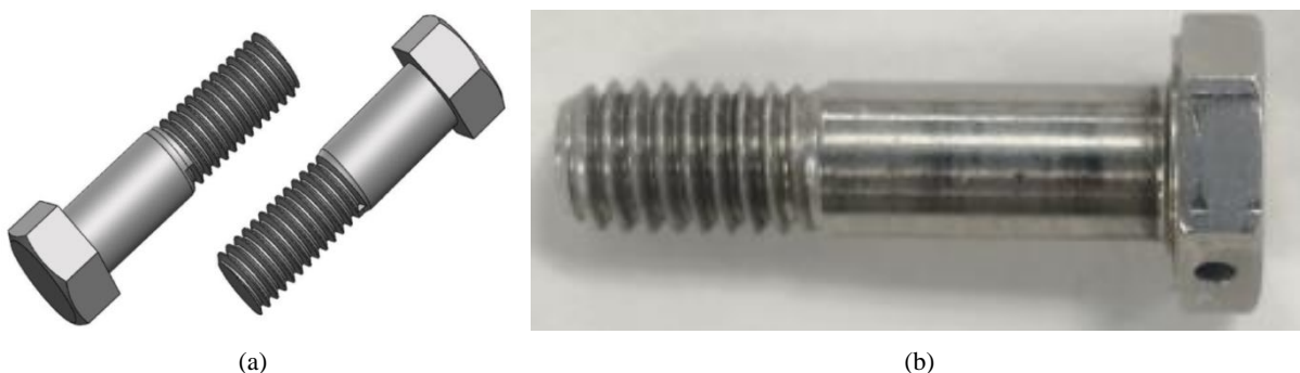
Figure 4. (a) Hexagonal bolt 3D model for to prepare the specimen by WEDM and (b) Bolt specification [27].
