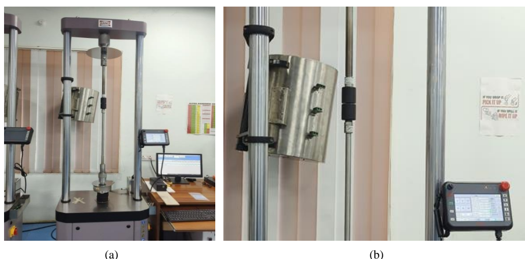
Figure 12. (a) Creep experimental set up (MIC_MT Lab) and (b) Mount the specimen.
