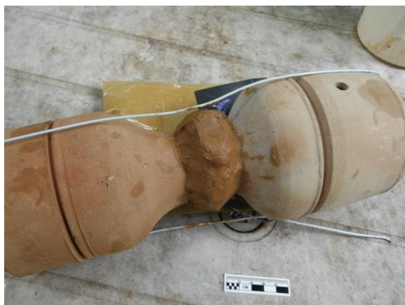
Figure 15. Double-ceramic testi-kabab retort with clay seal, vent to right.
