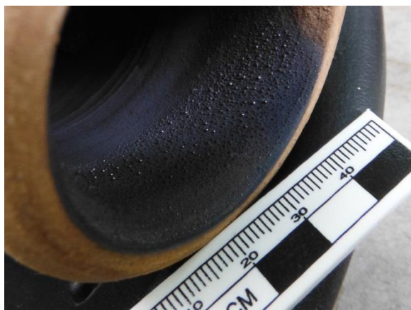
Figure 17. Mercury droplets in black mercury-rich residue (>100 ppm Hg) along rim of ceramic testi-kabab retort. For comparison, the blackened interior of a mercury smelter chimney at Karaburun, Türkiye had >400 ppm Hg. The sooty material consists of chlorides and sulfides of mercury and droplets of mercury [25]. And, at the mercury retorts at New Almaden, California this black sooty residue was scraped and removed to obtain additional mercury [11].
