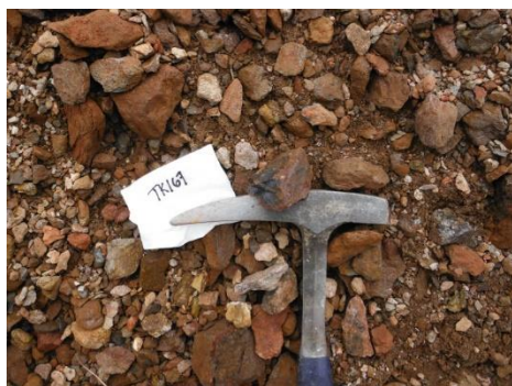
Figure 9. Halaköy Şubesi loading dock tailings from which a sample with 84 ppm Hg was taken (Table 1; sample TK167).
