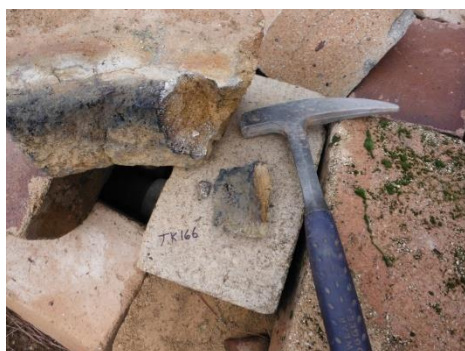
Figure 10. Halaköy Şubesi smelter stack scoria with 1.29 ppm Au, 7 ppm Ag, and 1272 ppm Sb (Table 1; sample TK166).
