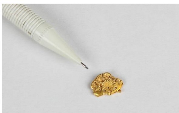
Figure 11. Anthropogenic gold nugget from Puerto Maldonado, Perú showing sponge-like texture resulting from burning (Spanish, refogado ) the mercury-gold amalgam to volatilize the mercury.
