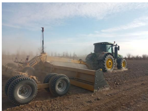
Figure 1. Laser land leveling in the "Ibrahim-Farida" experimental field.
