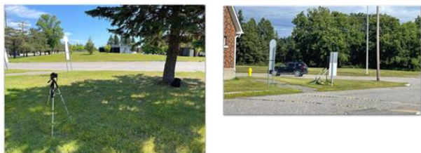
Figure 6. Camera mounted on a stand at the entrance of parking lot (LHS). Strip-dowel assembly plastered to the pavement's surface (RHS).
