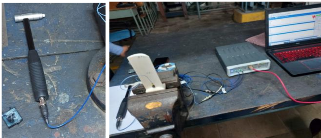
Figure 3. Tear drop type of accelerometer (make: PCB Piezotronics, Model 352C22), Instrumented impact hammer and the instrumentation set up comprising of (a) and (b) together with Multi-channel Data Acquisition System.
