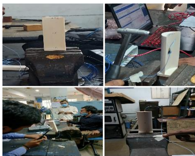
Figure 5. Testing using Impact hammer for giving force and to measure response by an accelerometer.
