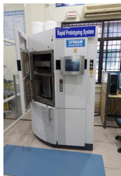
Figure 1. The dimensions of the blade and 3D Printer (Rapid Prototyping Machine, Formiga 100) used for manufacturing the blade (Make: EOS GMBH/Germany).
