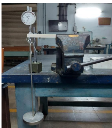
Figure 6. Bending test of cantilever blade.
