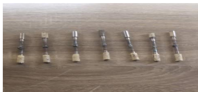
Figure 1. Tensile test specimens.
