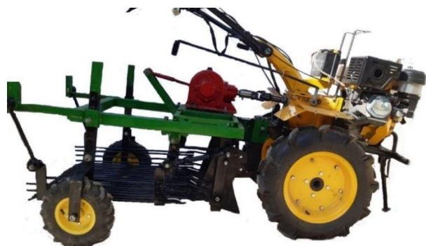
Figure 2. Scheme of aggregation of a small-sized potato digger with a walk-behind tractor.
