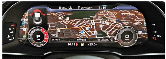
Figure 3. A digital dashboard is capable of displaying much more information than traditional analogue dashboards. Drivers can set up several appearances and choose the one that suits them best. Dashboard of an Audi Photo R. Rak
