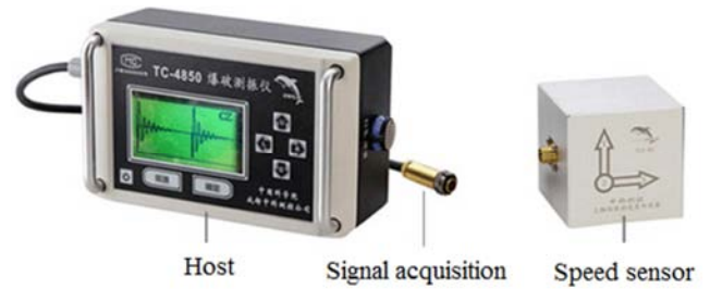
Figure 6. The measurement system of blasting vibration.
