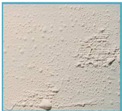
Figure 17. Solvent Blistering.
