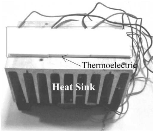
Figure 7. Cool air production system from thermoelectric.
