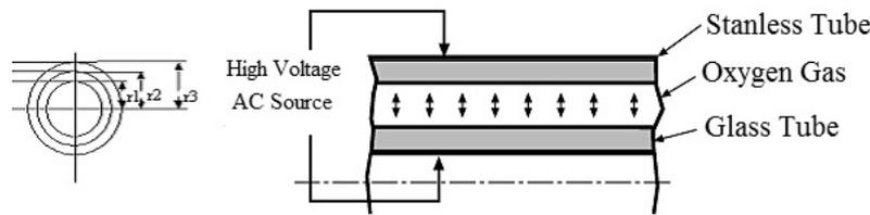
Figure 2. The structure of ozone tube.
