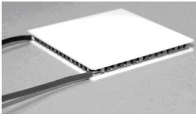
Figure 4. Thermoelectric /Peltier cooling (12V<sub>dc</sub> 40W).
