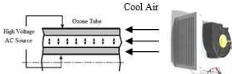
Figure 6. The connecting of ozone tube and Cool air production system by applied thermoelectric.
