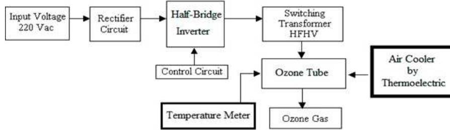
Figure 1. Block diagram of ozonizer using cool air production system.
