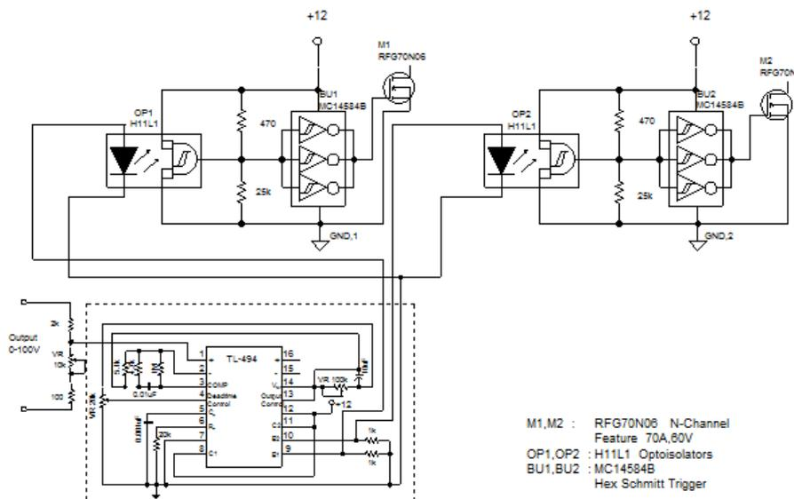
Figure 3. HF-HV switching power supply circuit using half-bridge inverter.
