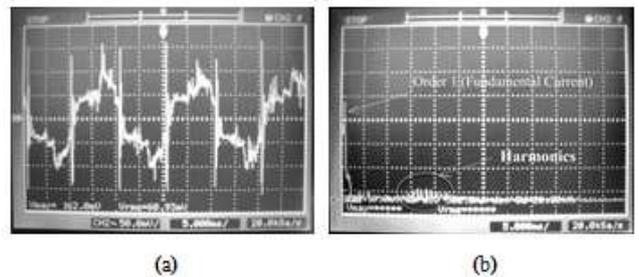
Figure 8. (a) Input current signal and (b) Input harmonics current of DC switching power supply 12V 100A of cool air production system from thermoelectric.
