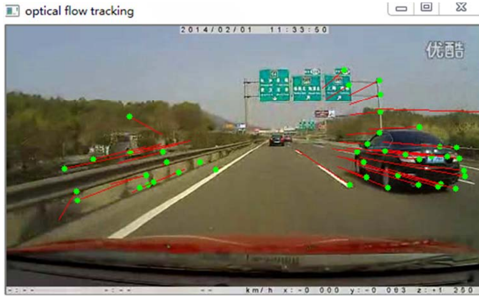
Figure 2. Optical flow detection.
