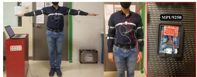
Figure 2. The experimental setup using five MPU9250 IMUs mounted on the body in the LASSENA laboratory.
