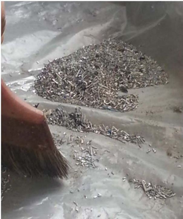
Figure 7. Connectors and slot connectors' weldings separated from their polymeric capsules and pins. Source: the authors.
