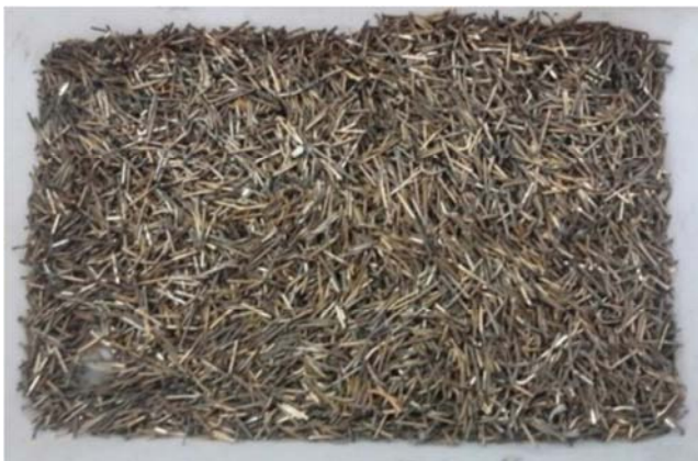
Figure 8. Liberated pins without welding tips of Pb/Sn and/or Sn/Ag/Cu. Source: the authors.
