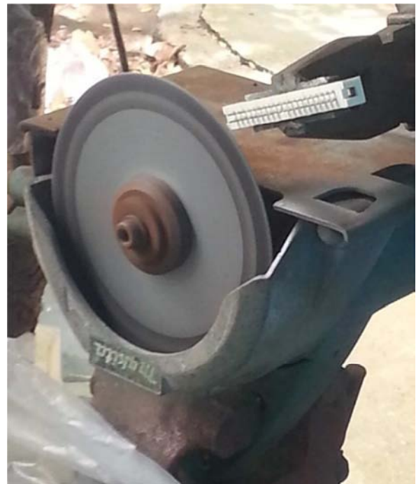
Figure 6. Saw machine used upside down along with an especial adapted tool (indicated with arrow) to hold the slot connector aiming at taking out the weldings of Pb/Sn and/or Sn/Ag/Cu. Source: the authors.
