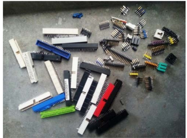
Figure 2. Polymeric encapsulations of motherboards’ connectors, slot connectors, and PCBs’ connectors along with its gold-rich pins. Source: the authors.
