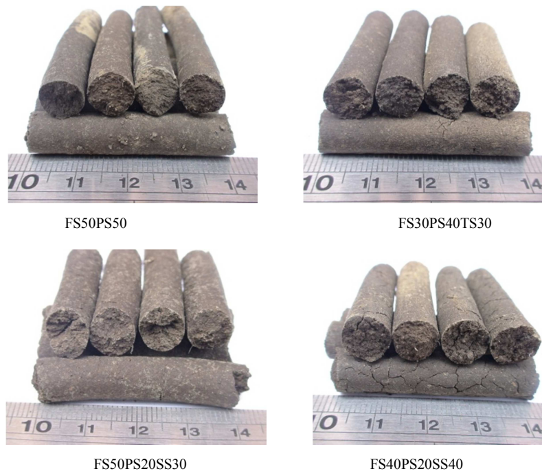
Figure 2. Appearance of industrial sludge biofuel briquettes.
