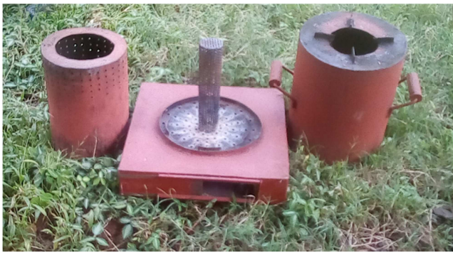
Figure 1. Main Components of a Stove.
