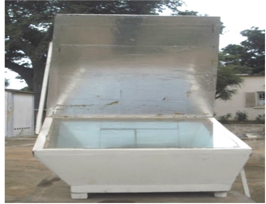
Figure 1. Solar cooker hot-box inclined lateral faces.
