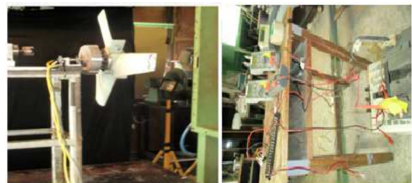
Figure 9. Testing the wind electric generator for electricity production
