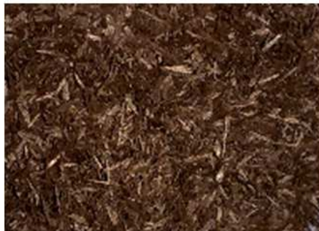
(c) Pretreated at 152°C, 5 bar, 45 min
