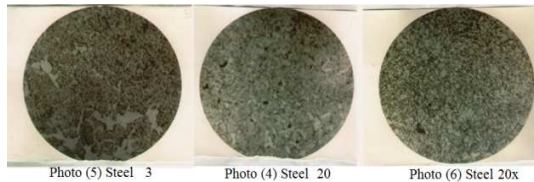
Photos show diffusion of carbon by wax from the surface to the steel core
