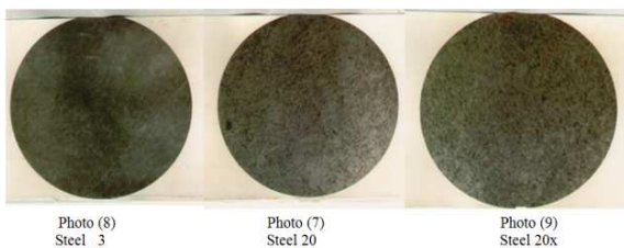
Photos show microstructure of carbonized layer by kerosene
