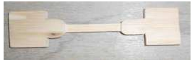
Figure 6. Geometry of the tensile test piece.
