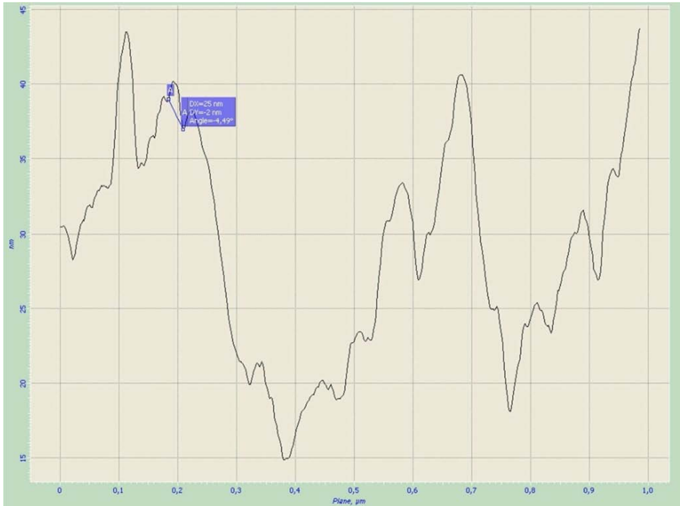
Figure 7. Surface relief of the Pb-VCT sample with vacancy cluster tubes images. The characteristic surface scales are determined using a power spectrum (Fourier analysis), Femtoscan online software applied
