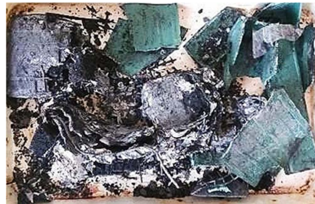
Figure 4. The Impact Crushing Effect of Plates of Spent Lead-Acid Batteries.
