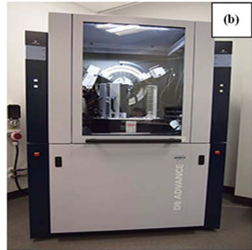
Figure 3. (a) True density measuring apparatus, (b) XRD machine.
