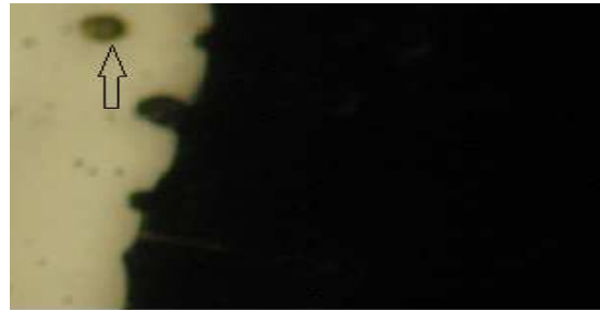
Figure 4: Optical image of inkjet-printed copper film showing absence of coffee stains and voids. However, satellite drops are clearly evident.
