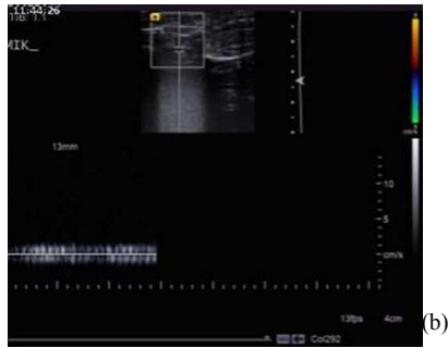
Figure 5. Spectral signal related to (a) glass and (b) magnet pieces was determined by spectral Doppler ultrasound imaging.
