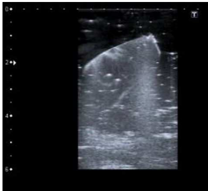
Figure 1. Remarkable reverberation artifact related to bullet in jelly were revealed.
