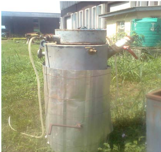
Figure 2. Locally made biogas digester.
