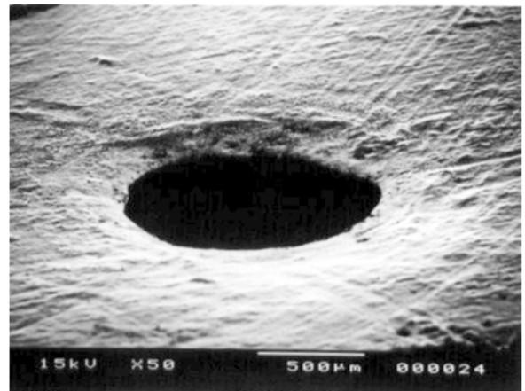
Fig.12. SEM Micrograph of machined micro hole (20 g/l elect. conc., 5V m/c voltage, 20% duty ratio and 2000 \mu sec pulse period).
