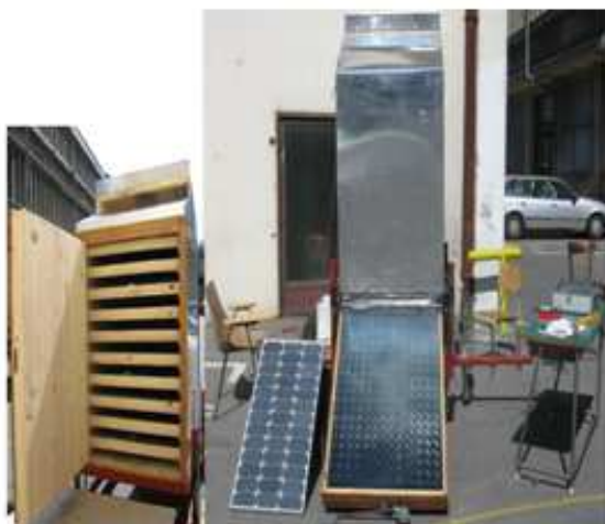
Fig 2. Prototype of one module of “MUECHAS” the solar dryer
