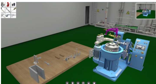
Figure 10. Virtual disassembly rendering of marine oil separator.
