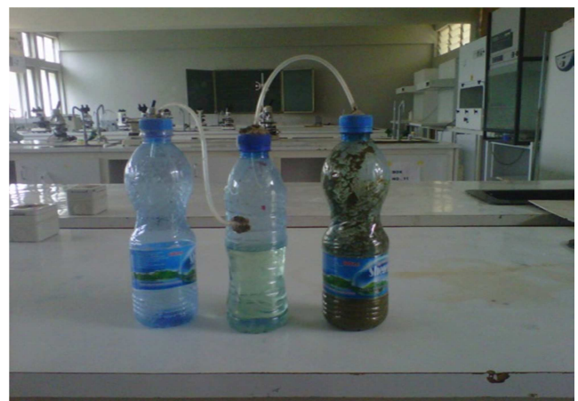
Figure 1. Arrangement of the digesters.
