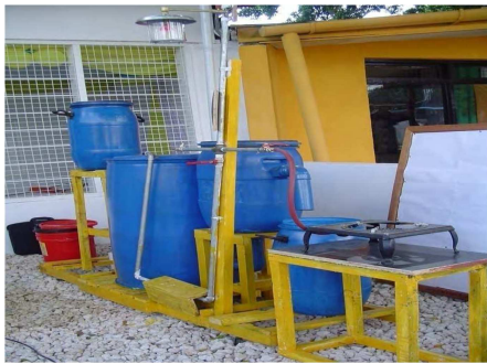
Figure 3. A biogas plant using plastic containers made by DIT [30].
